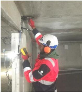
Fig. 4. Rebar electrical continuity test
